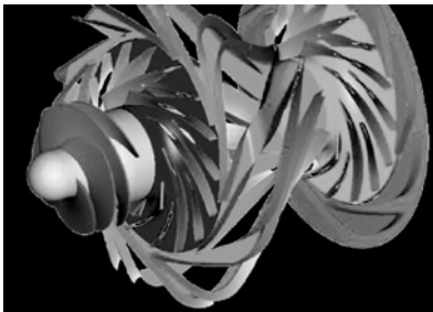
(e) Computer model of the liquid hydrogen pump of the VULCAIN engine of the European launcher ARIANE 5.
